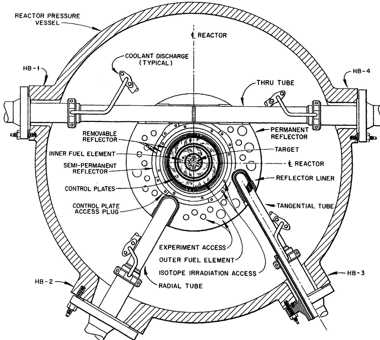
Fig. 5. Cross section of HFIR at core centerline.
