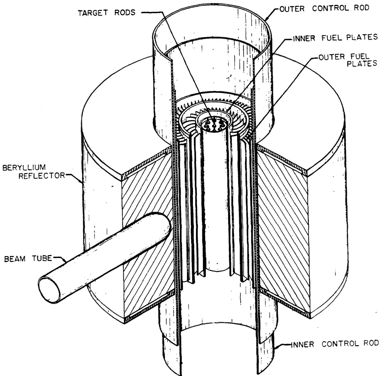
Fig. 3. Schematic of High Flux Isotope Reactor core.
