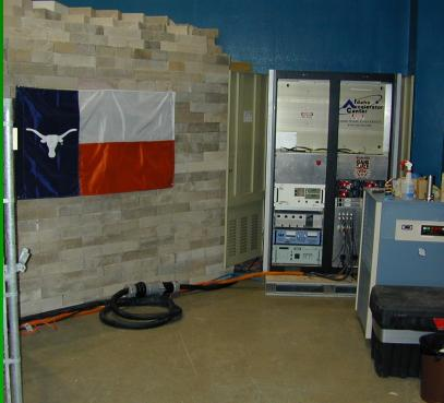
Linac power supplies, vacuum systems and main chiller Note: large extension cord
