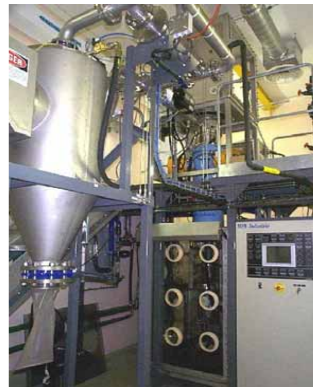
CVD line TRISO particle coating
