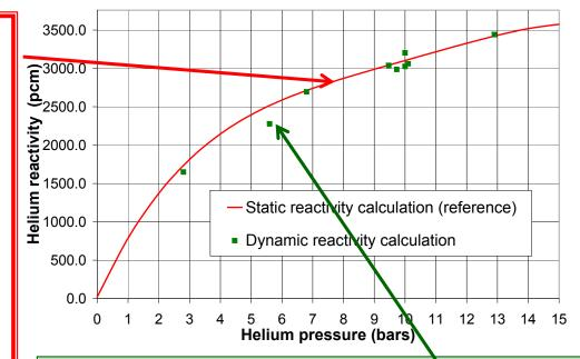
Dynamic Calculations (using  $\beta_{eff}$ ,  $\Lambda_{eff}$ , Doppler) Experimental power bursts obtained in the past can be interpreted by inverse kinetics. One can determine the injected helium reactivity for different tests (performed at different helium pressure)  $\rightarrow \rho^{3He} = f(Pressure)$
