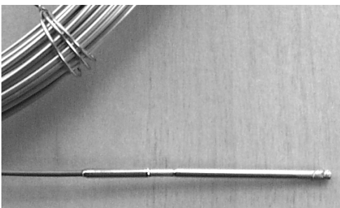
Fig. 7. Fission chamber with integrated cable (1.5mm diameter)
