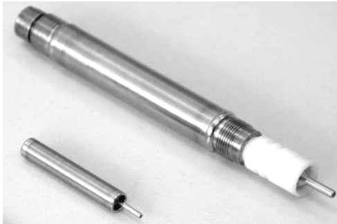
Fig. 6. CEA fission chambers (4mm and 8mm diameter)
