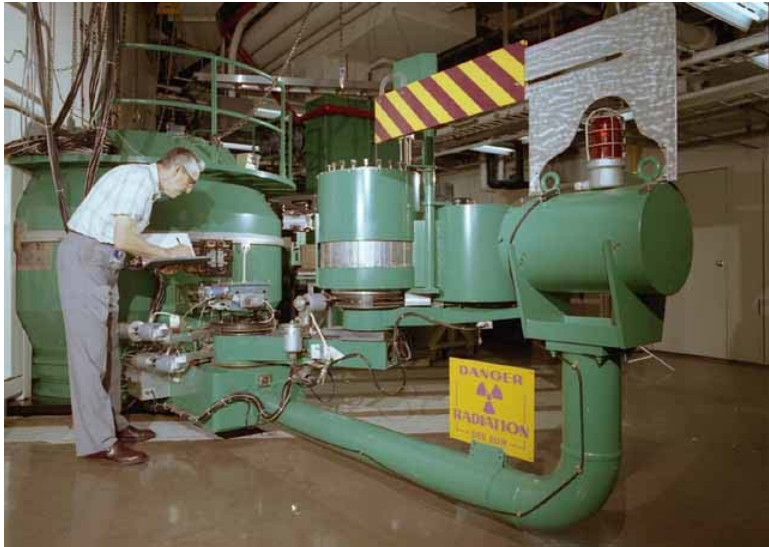
A triple-axis spectrometer on one of HFIR's four neutron beams
