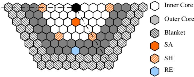
Fig. 2. Radial configuration of core.
