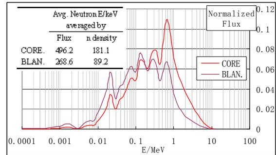
Fig. 4. Core and blanket neutron spectrum of CASE A.
