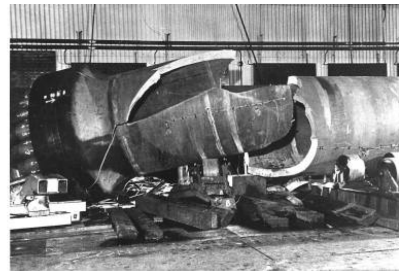
CATASTROPHIC FAILURE OF PRESSURE VESSEL DURING HYDROSTATIC TESTING; DUE TO IMPROPER POSTWELD HEAT TREATMENT
