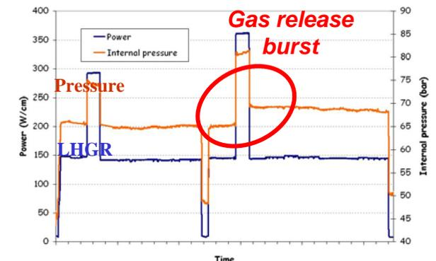
On-line measurement of the fuel rod pressure during power ramps in the REMORA-2 experiment
