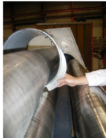
Photo 3: Post-forming inspection using a template
