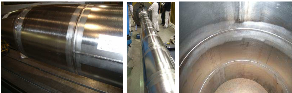
Photos 12 to 13: Plasma welds (external, entire assembly, internal)
