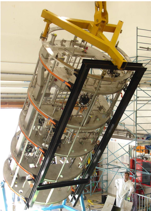
Fig. 3. The basket : support structures for the new CABRI water loop.
