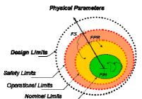
The Pilot Functions (FPI) & the Preventive Function (FPR) are implemented inside the operational I&C systems (mostly CS automation system) to maintain the reactor within operational limits.
