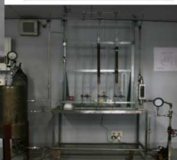
CLOE : feedthroughs, flow amplifier, chemistry control ; sample holder, loading system, DCPD,...
