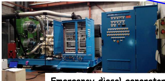
Emergency diesel generator (tested on a shacking table)
