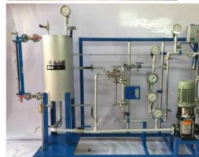
CLOE : feedthroughs, flow amplifier, chemistry control ; sample holder, loading system, DCPD,...
