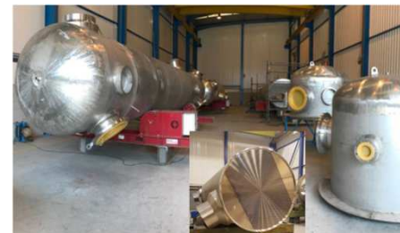
Heat exchangers (primary/secondary system)
