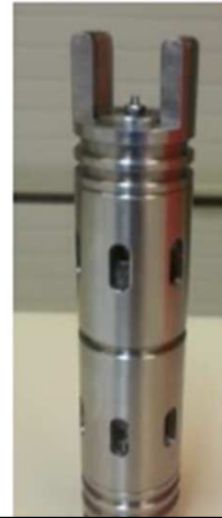
"Two-way Filter" (patented), dedicated to trap Na-K oxides and hydrides
