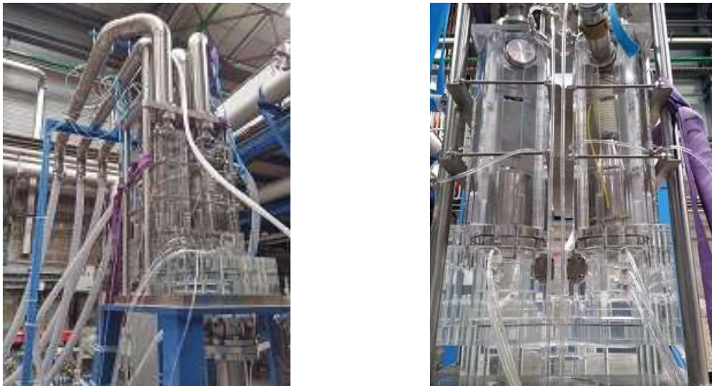
Figure 7 : C4 sector water box mock-up (in Plexiglas)
