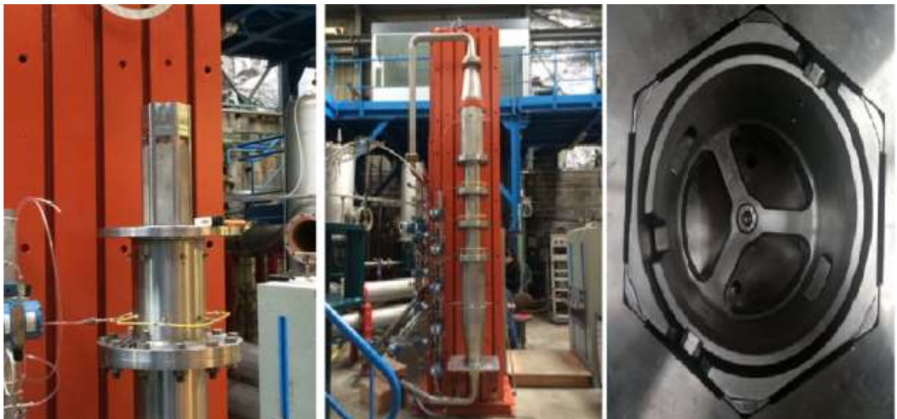
Figure 6 : Beryllium block mock-up (hexagonal shape)
