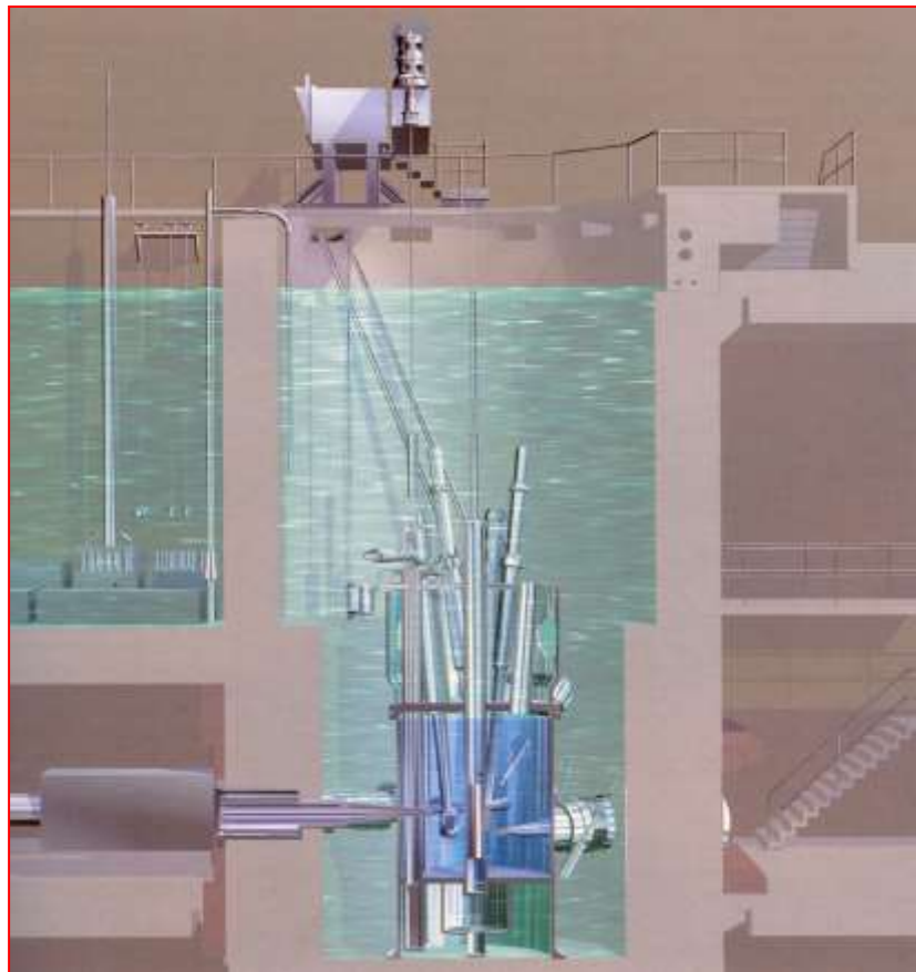
Fig 1: FRM II reactor pool and moderator tank (dark blue) with some key components
