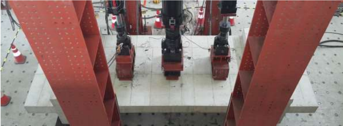
FIG. 5. Static loading test (original condition)
