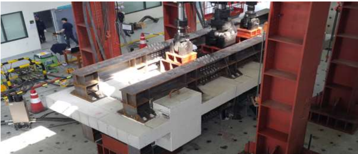
FIG. 6. Static loading test (reinforcing with built-up section)
