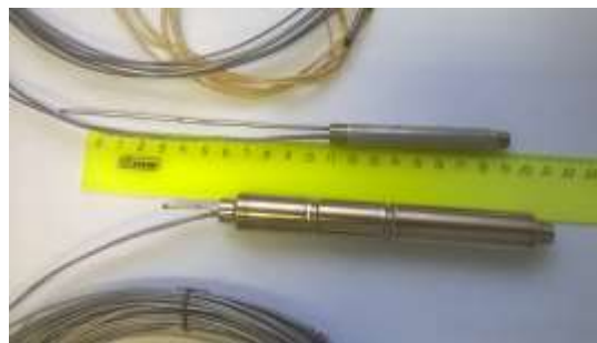
FIG. 4. Differential transformer of a high-temperature gage to measure gas pressure under the cladding.
