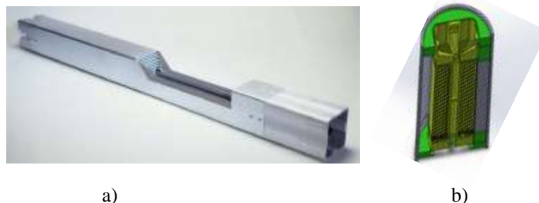
FIG. 20. IRT-3M LTA (a) and experimental channel with LTA (b).
