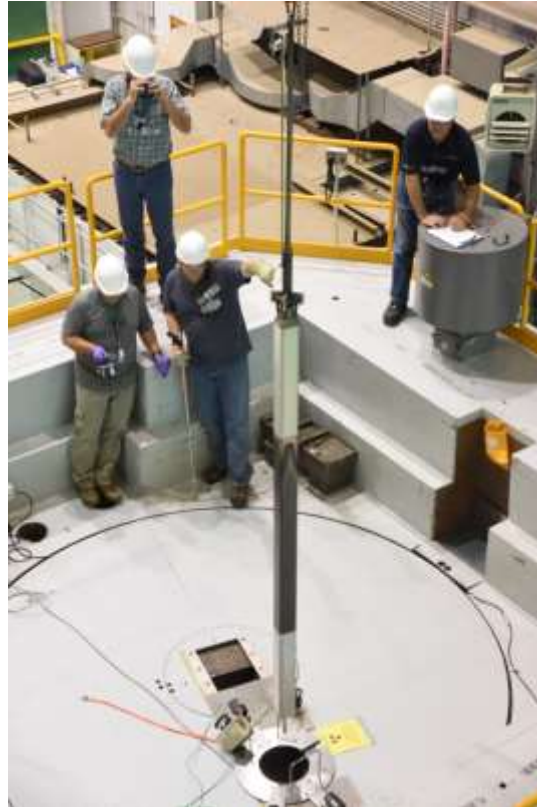
FIGURE 1. TREAT Fuel Assembly Lift and Inspection
