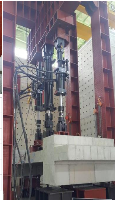
Static loading test (Left : Original wall, Right : Reinforcing with built-up section)
