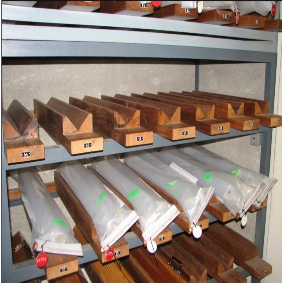
Close-up View of the Fuel Assembly Cradles
