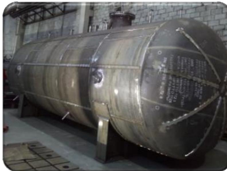
Drain tank of the primary circuit
