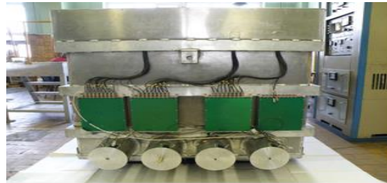
Neutrino detector for NEUTRINO-4 Experiment
