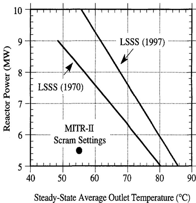
Figure 1. Comparison of the Calculated LSSS using MULCH-II and the LSSS used in the MITR-II SAR.
