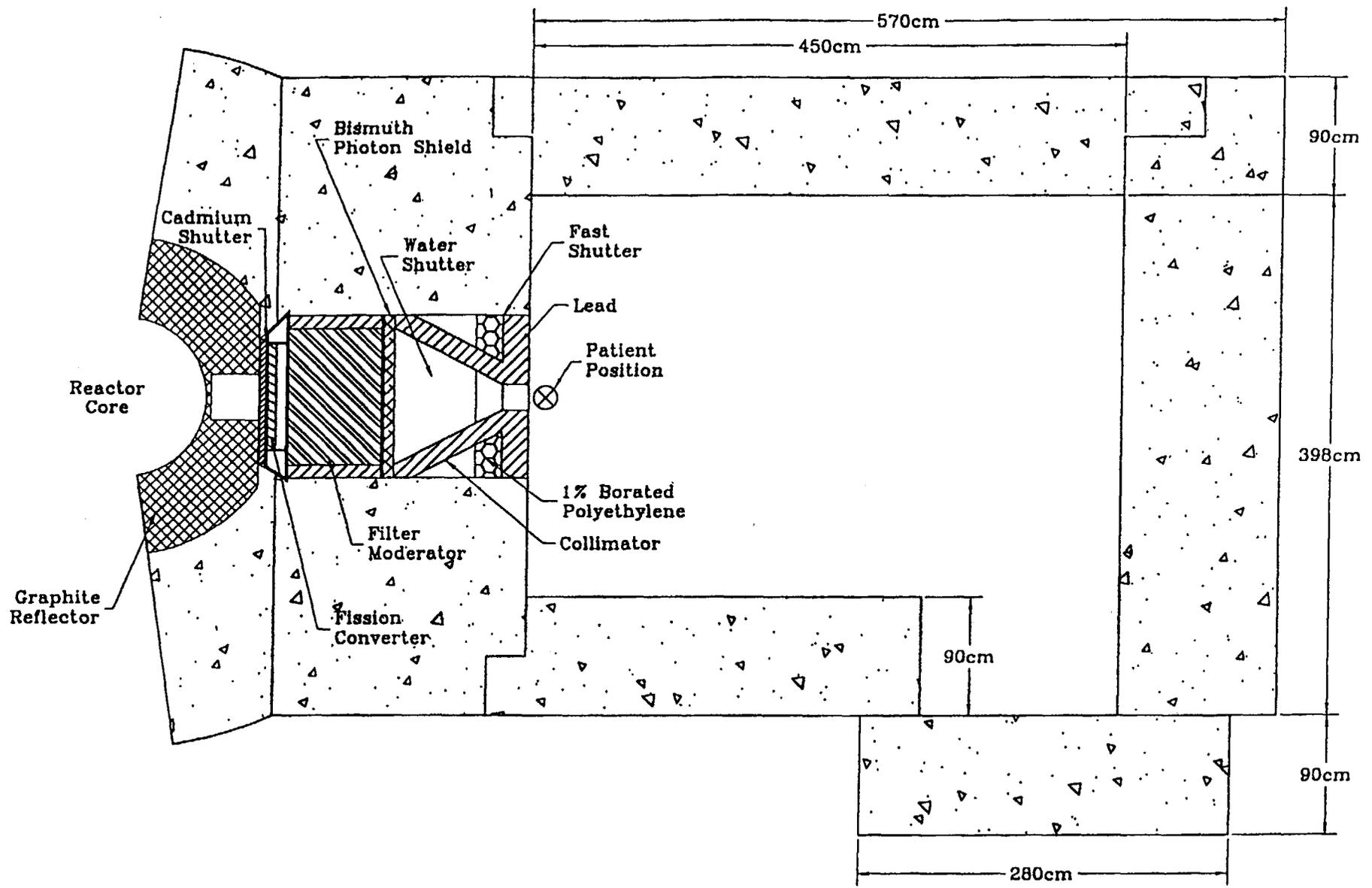
Figure 2. Top View of the Fission Converter Facility.
