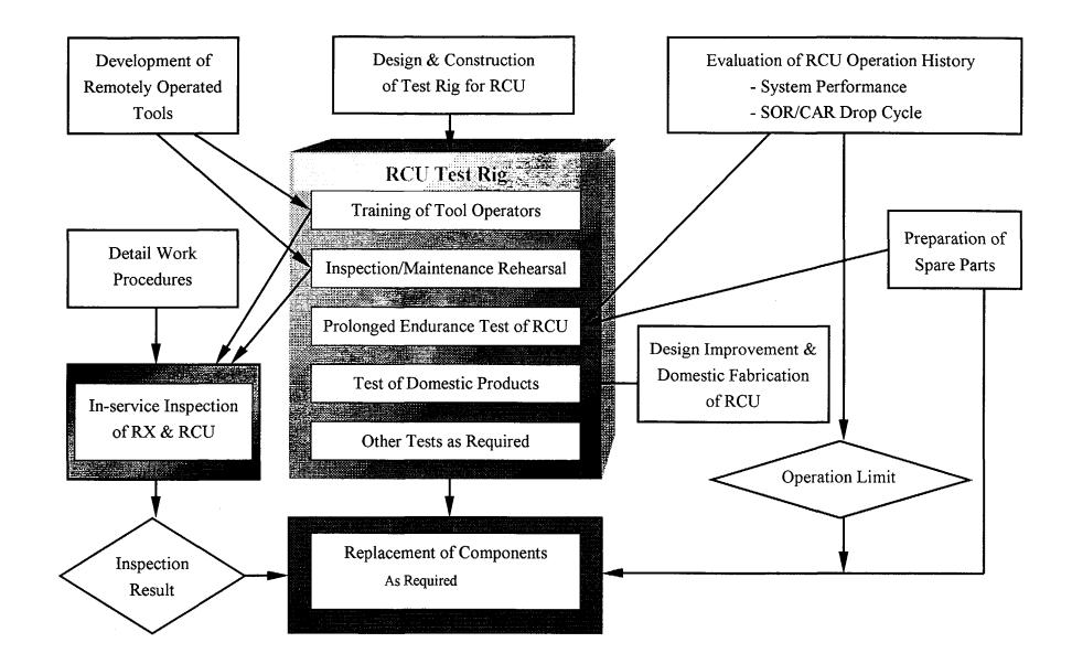
Figure 1. Flow Diagram for Inspection and Maintenance of Reactor and RCU
