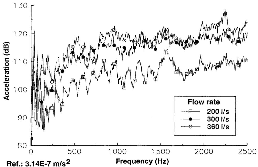
Fig. 4: Acceleration at the spherical seat
