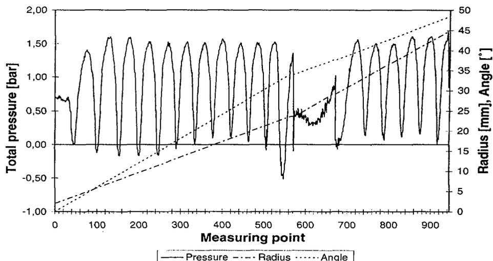
**Fig. 6: Total pressure at the outlet of the plate zone**
