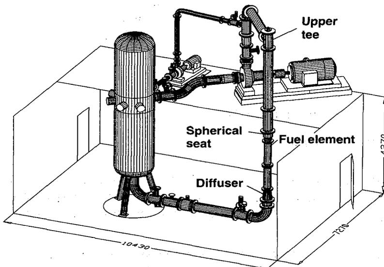
**Fig. 3: Test facility for the hydraulic and mechanical analysis of the FRM-II fuel element**
