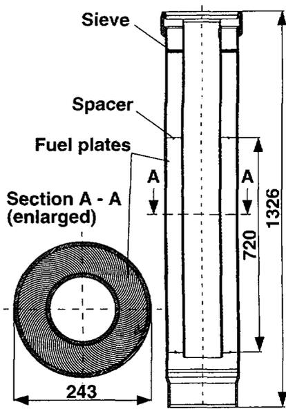
**Fig. 2: Longitudinal and cross section of the fuel element**
