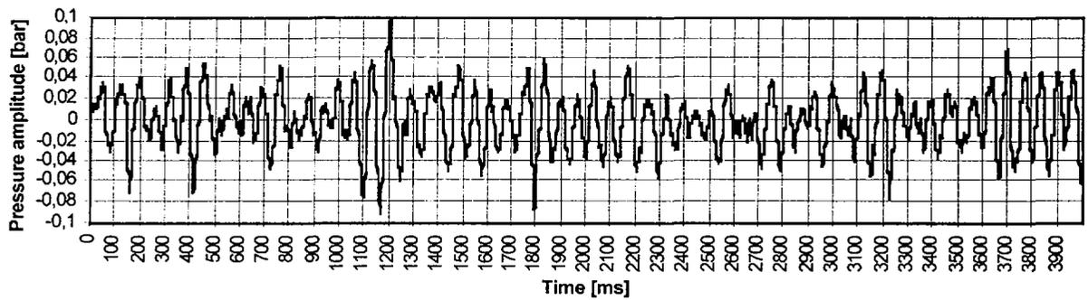
**Fig. 9: Maximum amplitudes of pressure pulsations after the transition from forced to natural convection at a dead loss of the cooling system**
