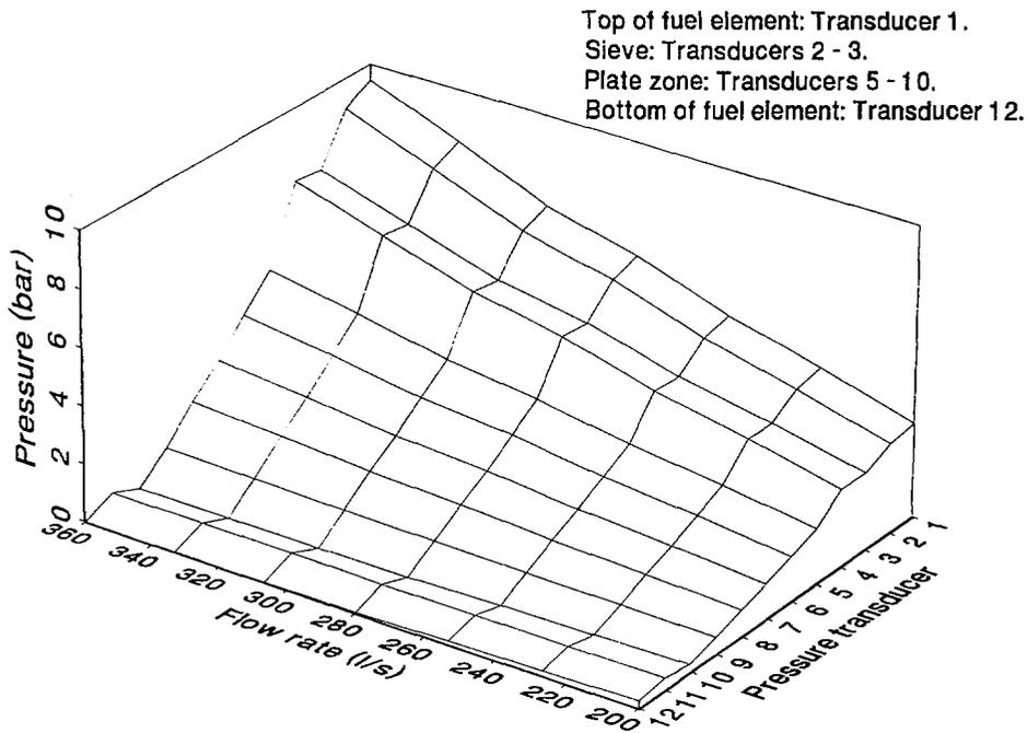
**Fig. 5: Pressure course inside the fuel element**
