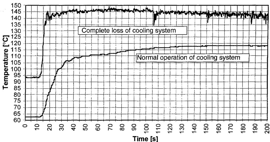
**Fig. 8: Wall temperatures at the upper part of the heated zone during the transition from forced to natural convection**
