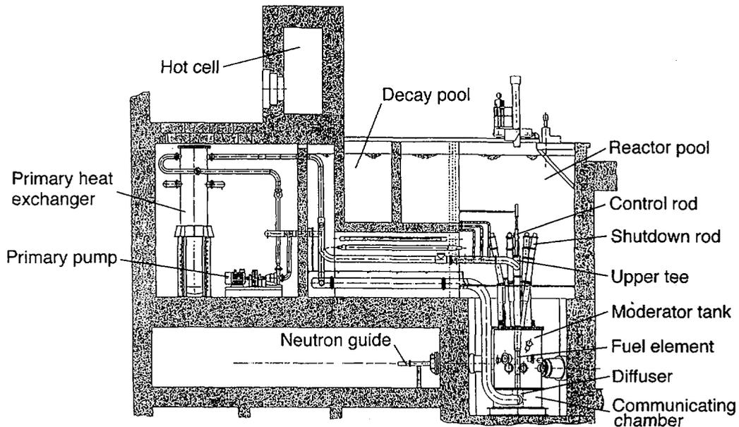
**Fig. 1: Sectional view of the FRM-II reactor building (Source: Siemens KWU)**
