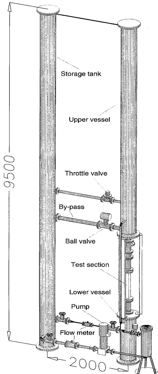
**Fig. 7: Facility to investigate the decay heat removal in the FRM-II**
