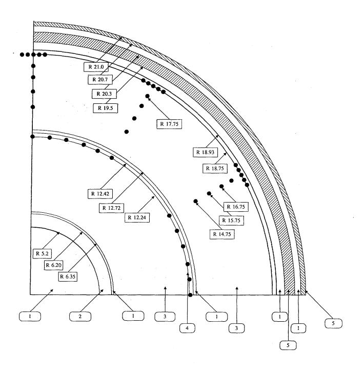
Fig.4. Burnable-absorber bar (BAB) coordinates
