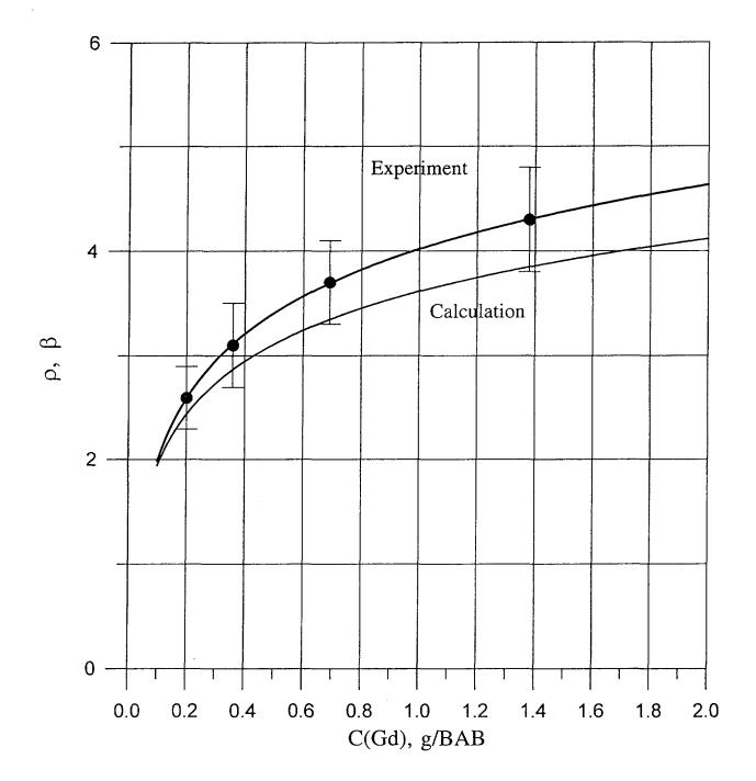
Fig.3. 144 BAB efficiency as function of gadolinium loading
