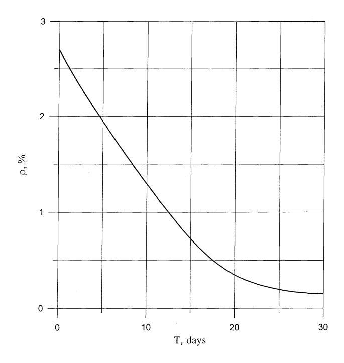
Fig.7. 144 burnable-absorber bar (BAB) reactivity in the PIK reactor calculated for an infinite cylinder
