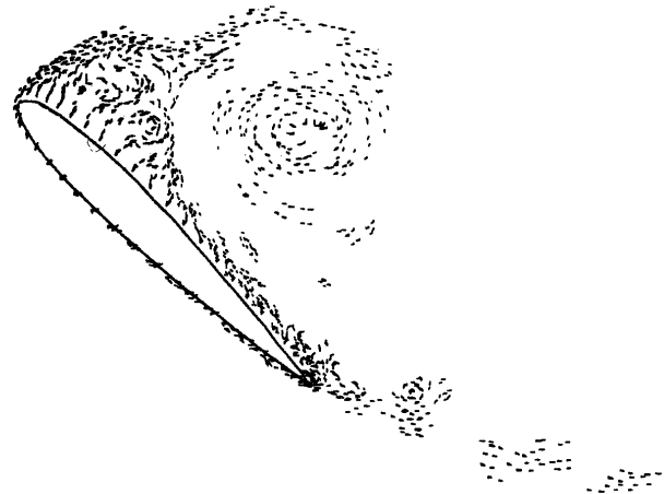
Fig. 8: Vortex shedding caused by flow separation.
