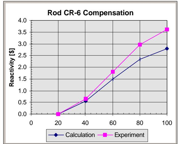
Figure 3: Calibration of CR's 1 and 6 for Core 2/98.
