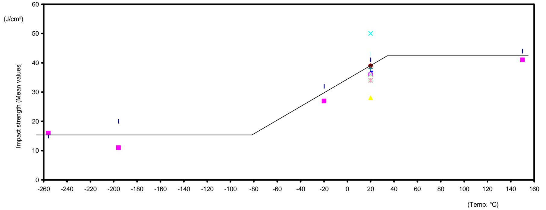
Figure 3: Transition curve of the impact strength for forgings
