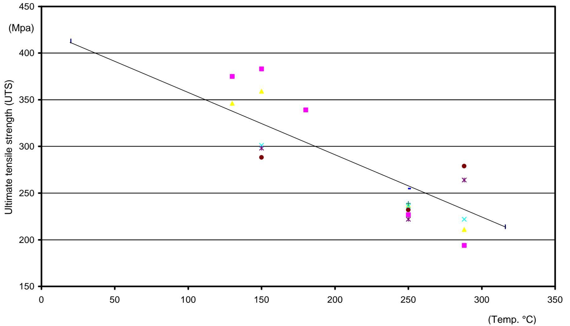
Figure 2: Ultimate tensile strength (UTS) of Zircaloy 4 forgings versus temperature
