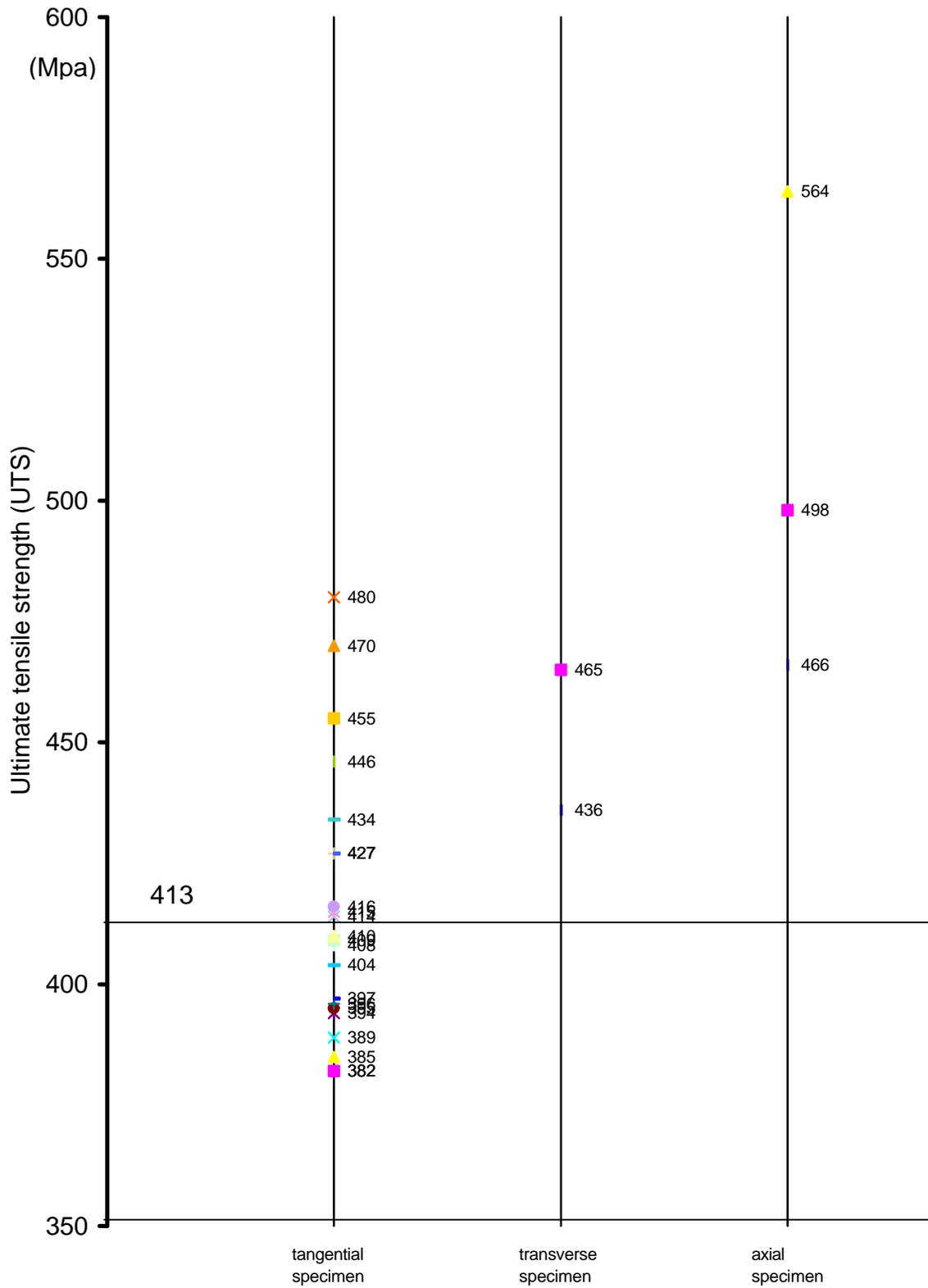
**Figure 1: Ultimate tensile test (UTS) at RT for the tangential, transverse and axial direction of forgings**
