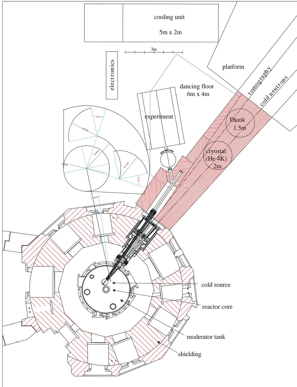
**Figure 2.** Plan view of the reactor core with the UCN source in beam tube SR4
