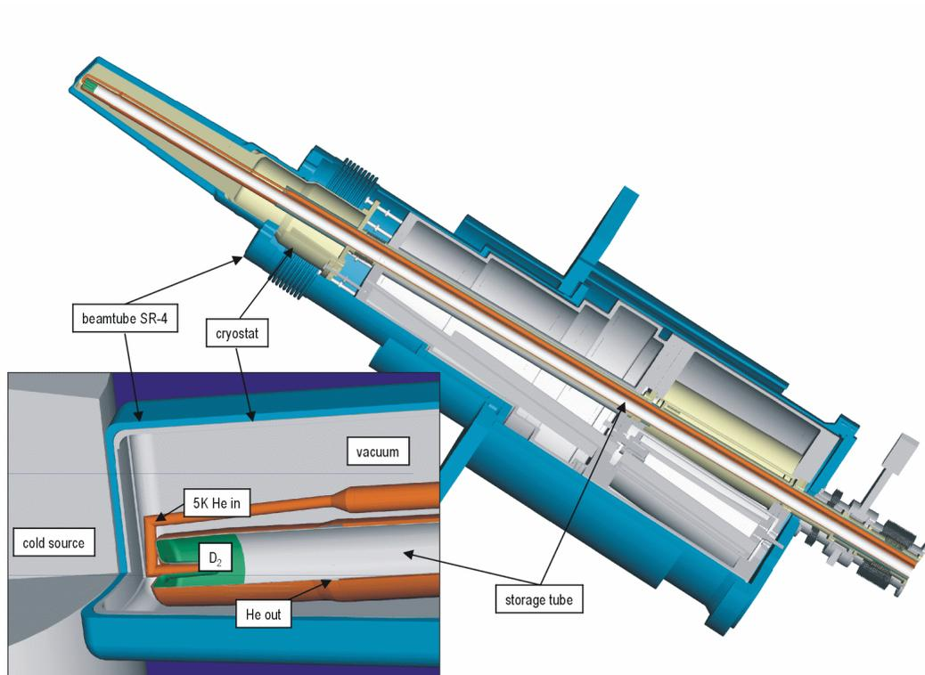
**Figure 3.** Cutaway view of the inner part of the beam tube SR4 with the Mini-D<sub>2</sub> UCN source.
