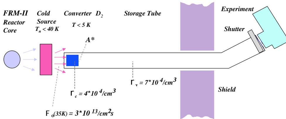
**Figure 1.** Scheme of the reactor-driven UCN source Mini-D<sub>2</sub>
