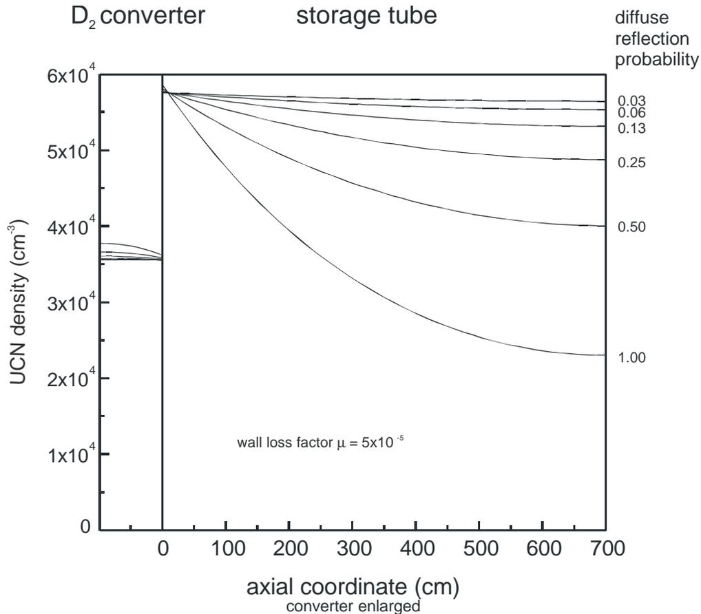
Figure 4. UCN density distributions along the axis of the converter and the storage tube.
