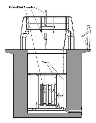
The present grids allow configurations up to 3500 fuel elements in an hexagonal geometry. Also serve as support for neutron detectors and thermocouples to measure the moderator temperature. The grids can be easily replaced by new ones changing, for example, geometry and pitch and keeping the other components unaltered.
