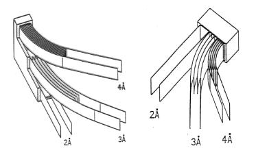
Fig. 4: Two types of beam splitters
