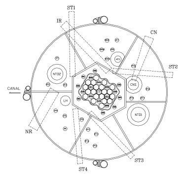
Fig. 1 Plan View of HANARO Core and Reflector
