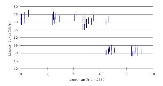
Fig. 4 Linear Power History of High-density U<sub>3</sub>Si<sub>2</sub> Mini-plate in HANARO
