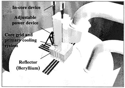
The primary circuit is closed to make it a real second barrier and to allow a pressurisation of approx. 5 bar at core outlet: the core has to be located in a pressurised tank.
