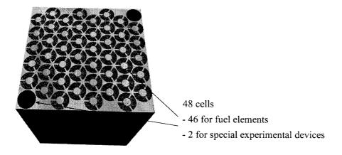
The core is arranged with a triangular lattice, in an aluminium rack, which is a part of the reactor tank.
