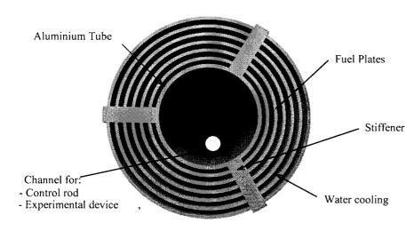
The fuel element is made of curved fuel plates, arranged in a cylindrical pattern. In the preliminary design, the fuel element has a row of six U-Mo- Al fuel plates bonded to three stiffeners. An aluminium tube protects the inner plate. Others designs are considered with silicide fuel, or with a larger fuel element.
