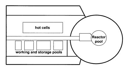
The pools are distributed in two nuclear buildings: one for the reactor, and the others for nuclear and experimental auxiliaries. In the second building, experiments are prepared in a working pool, and dismantled or measured in hot cells.
