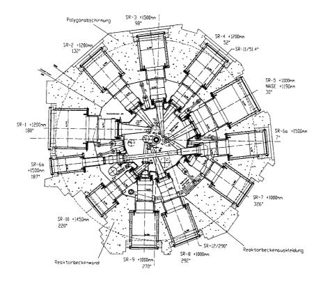
Inside the reflector tank the beam tube structures are shaped by the inner cones which are made of Alalloy with circular and rectangular cross sections. They are located in the region of maximum neutron flux (exception BT10), they are directly connected to the flanges of the reflector tank, their lengths are about 1.5 m (exception BT10) and their axes are directed tagentially to the core centre thus contributing to a low  $\gamma$ -noise at the experiments.
