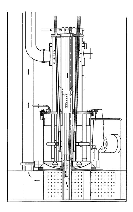
Fig.1 Longitudinal Cut View of CARR Core
