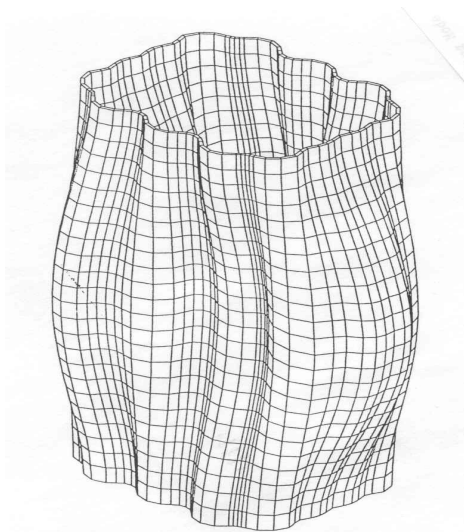
Figure 4. Deformation of Inner Shell
