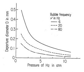
Fig. 6. Departure diameter as a function of system pressure.
