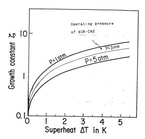
The growth rate becomes large with increase of super heat. The larger the nuclear heating of the moderator cell wall, the larger the super heat of liquid becomes. Thus the material and thickness of the wall should be designed reasonably. As bubbles are hard to grow so large under the higher pressure, the system pressure of 3 to 5 atm is recommended in practice. The departure diameter of the bubble is also depending on the system
