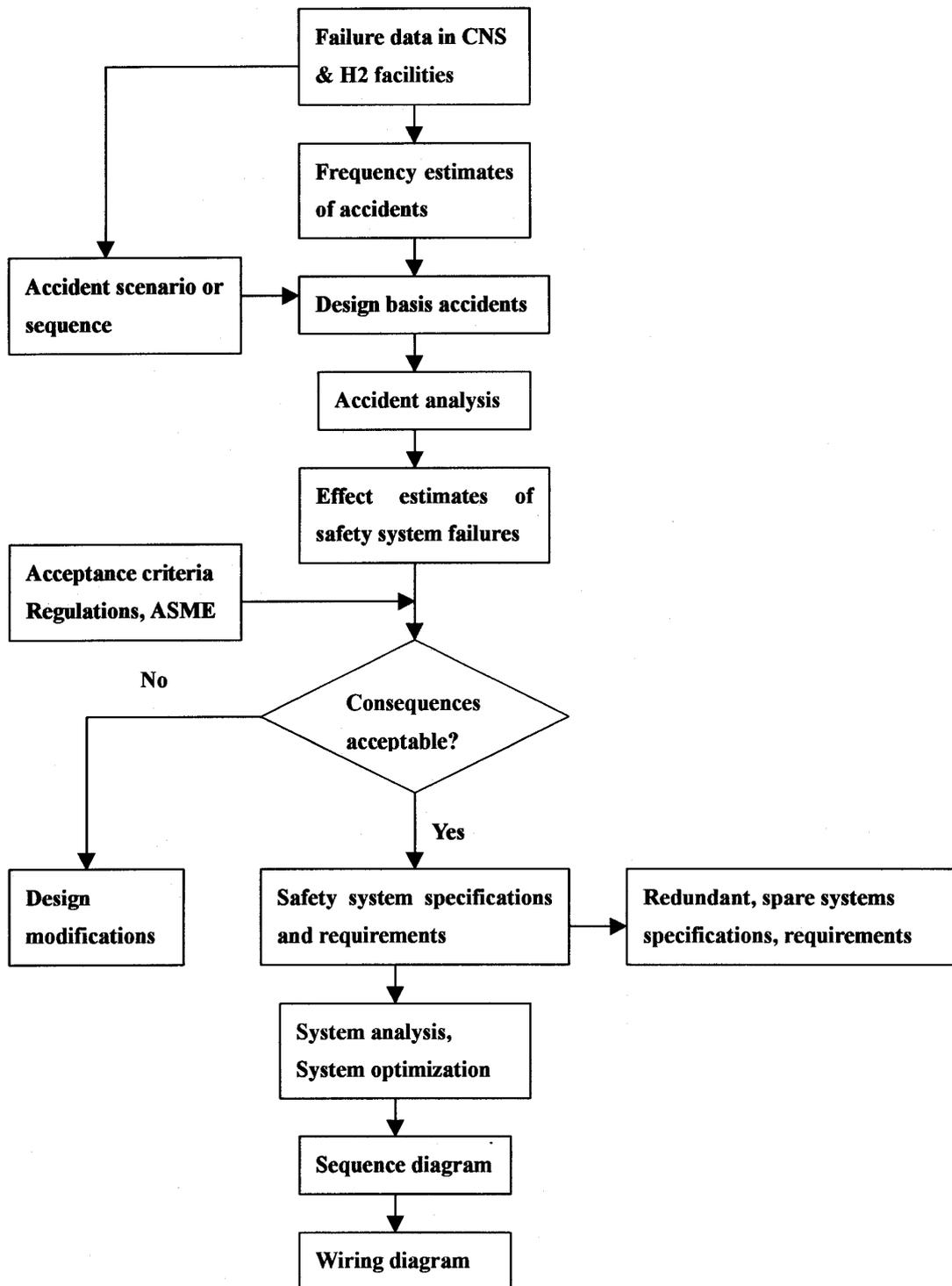
**Fig. 2. Safety system design flow chart of CN**
