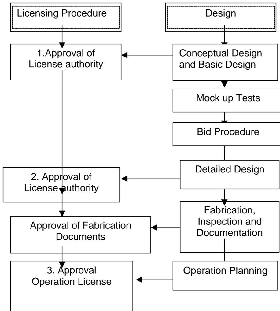
Fig. 1: Design guidance of cold neutron source.
