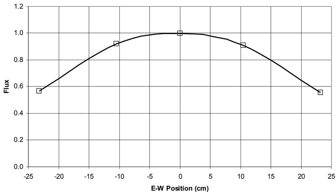
Figure 2b – FNR relative flux profile (E-W along the south guard plate)
