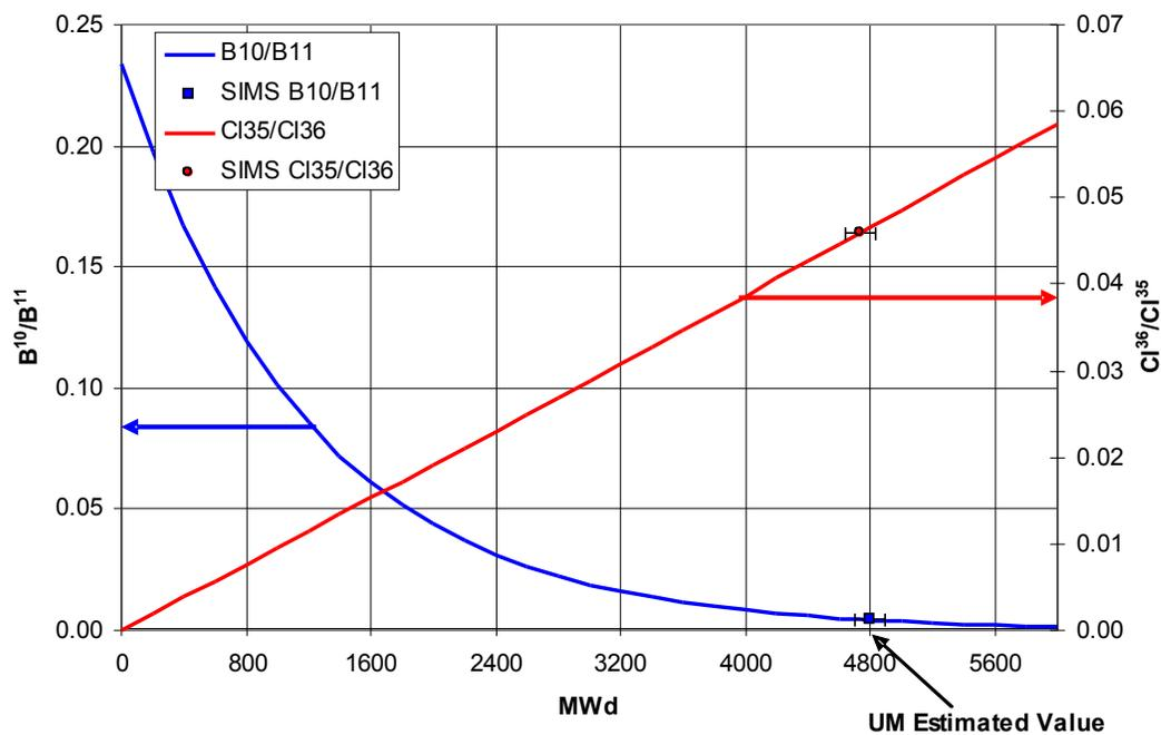
Figure 3 –  $B^{10}/B^{11}$  and  $Cl^{36}/Cl^{35}$  as a function of MWd at -23.2cm
