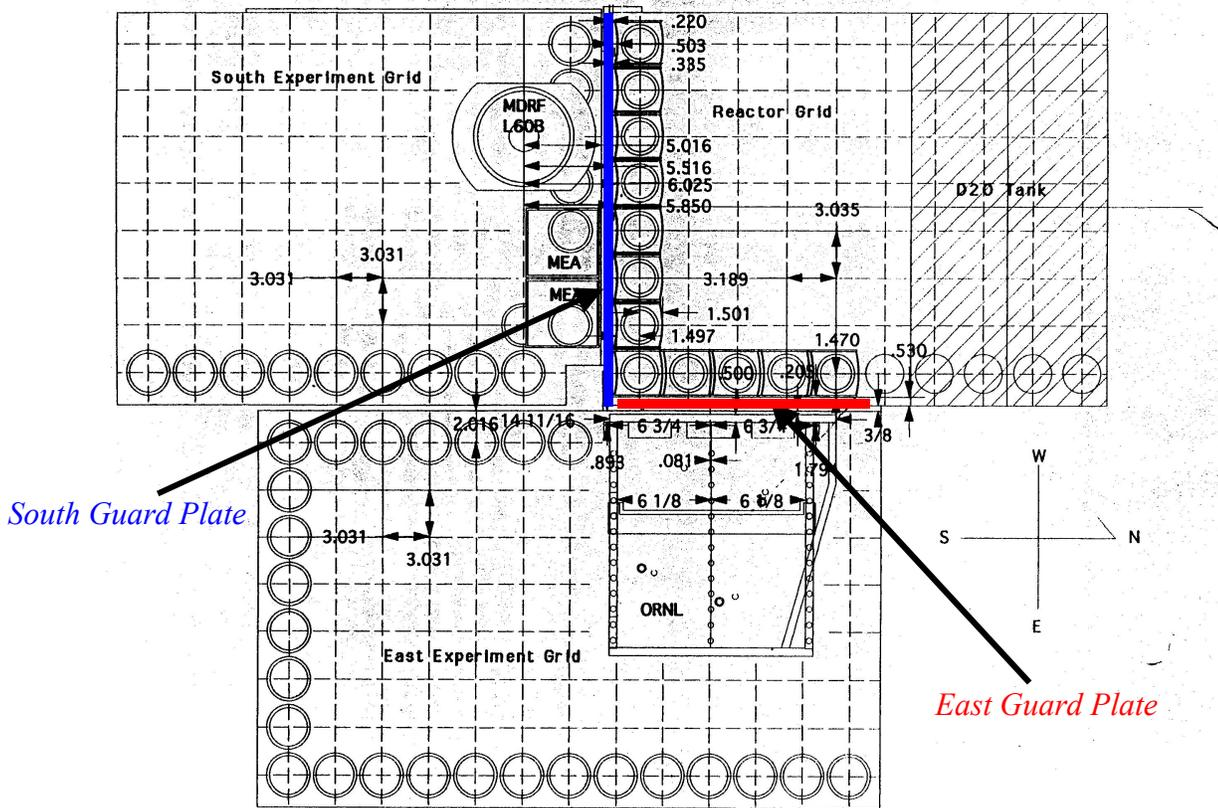
Figure 1 – FNR core/experimental grid layout (top view)
