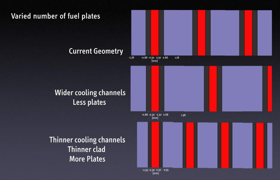
Variation of cooling channel, cladding and meat thickness (19.75% enriched, 70 cm )
