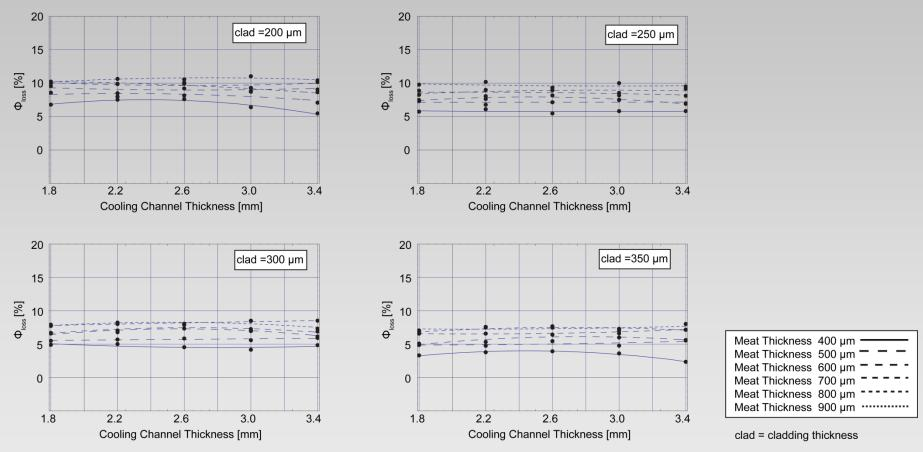
Increasing cooling channel thickness has nearly no influence on flux losses Reducing cladding thickness increases flux losses Increasing meat thickness increases flux losses (but less than at max position)
