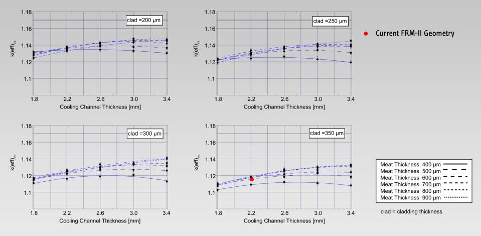
Optimum cooling channel thickness between 2.6 and 3.4 mm The more cooling channel thickness the more sensitive is k(eff) on the meat thickness
