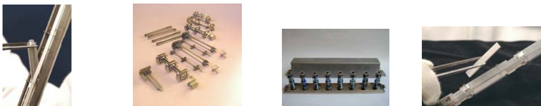
Fig. 4. Examples of CHOUCA loadings with various kinds of Candu or LWR samples.
