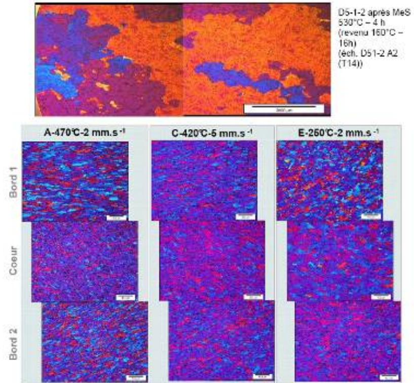
Microstructures obtained on Servotest samples in different conditions (T, strain rate)
