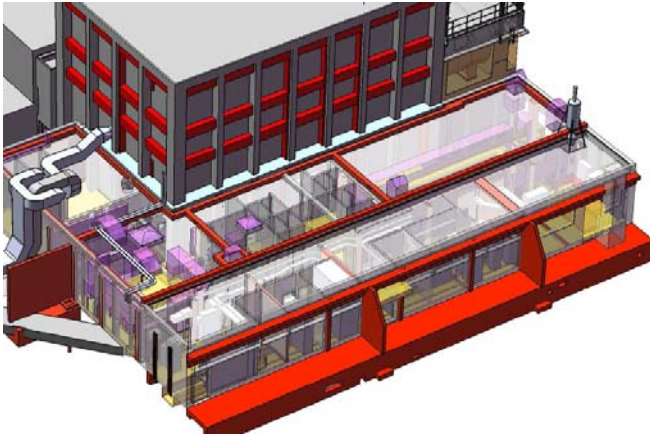
Fig 1 : CABRI main seismic reinforcement (in red)
