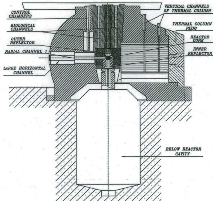
Figure 2 – TAPIRO Vertical Section
