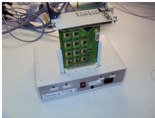
Fig 3. Testing of one PCB card developed for the safety system SS-I in a test unit connected to the computer
