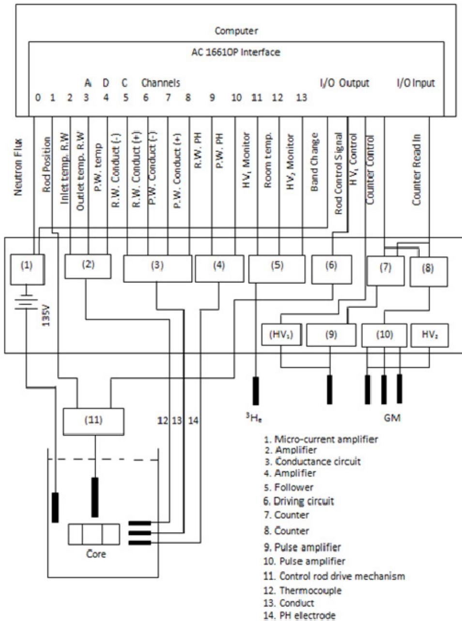
Figure 4.1 Hardware of the computer control system
