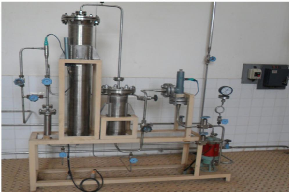
Fig. 4.10: Reactor water purification system
