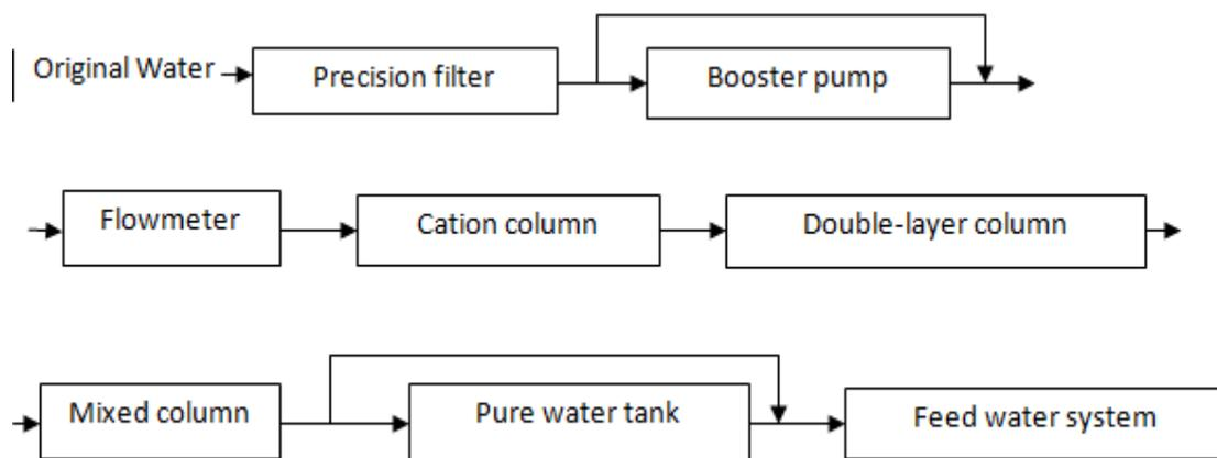
Fig.4.8. Flow chart of pure water processing
