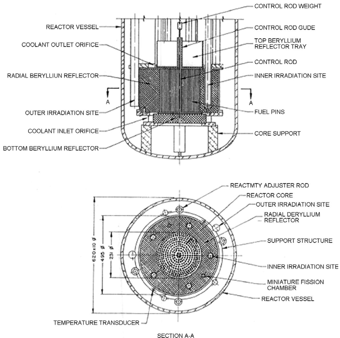
Figure 1 : The cross sectional view of GHARR-1 core
