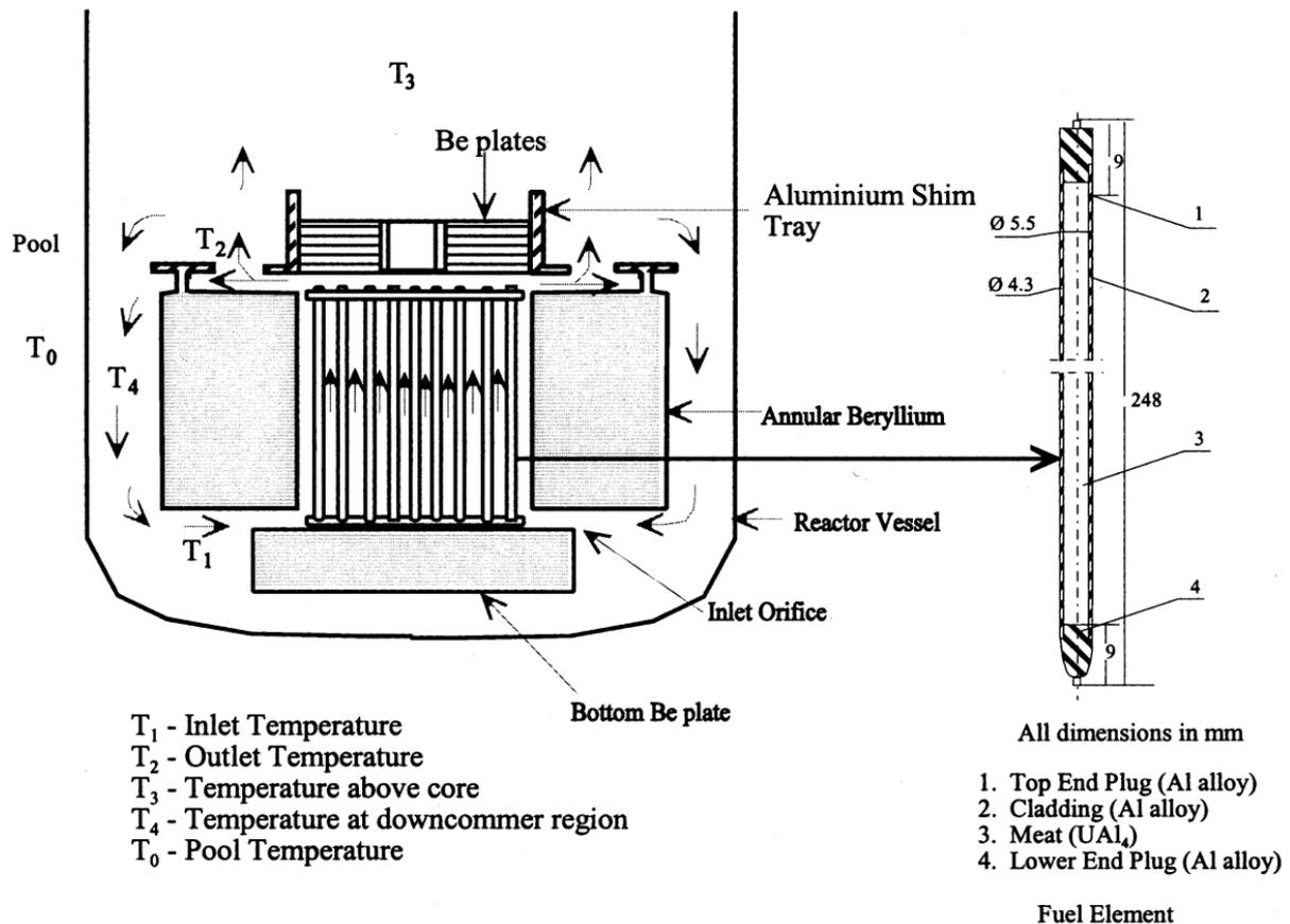
Figure. 2 Schematic diagram of the coolant flow pattern
