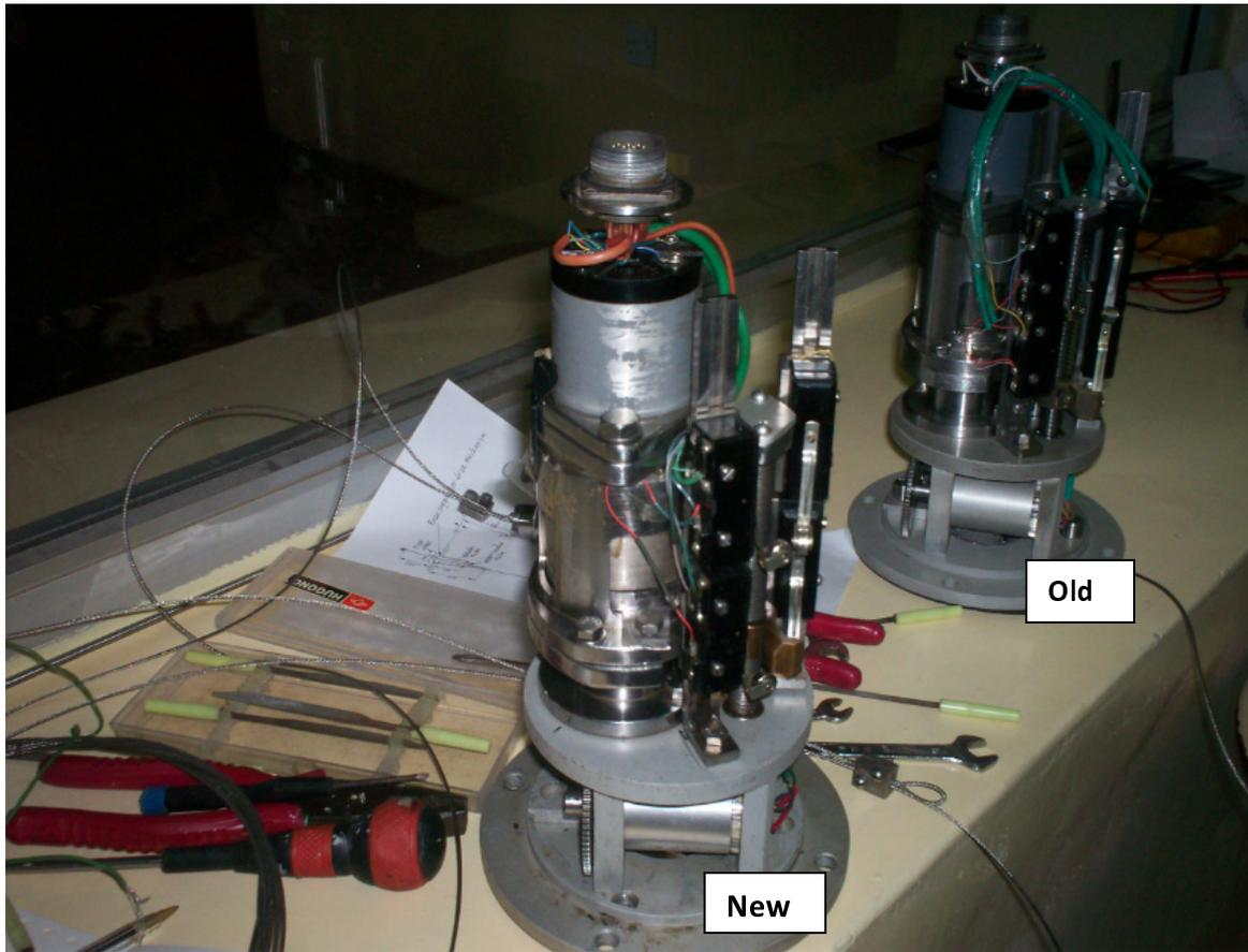
Figure 4.2. Old and New Control Rod Drive Mechanism
