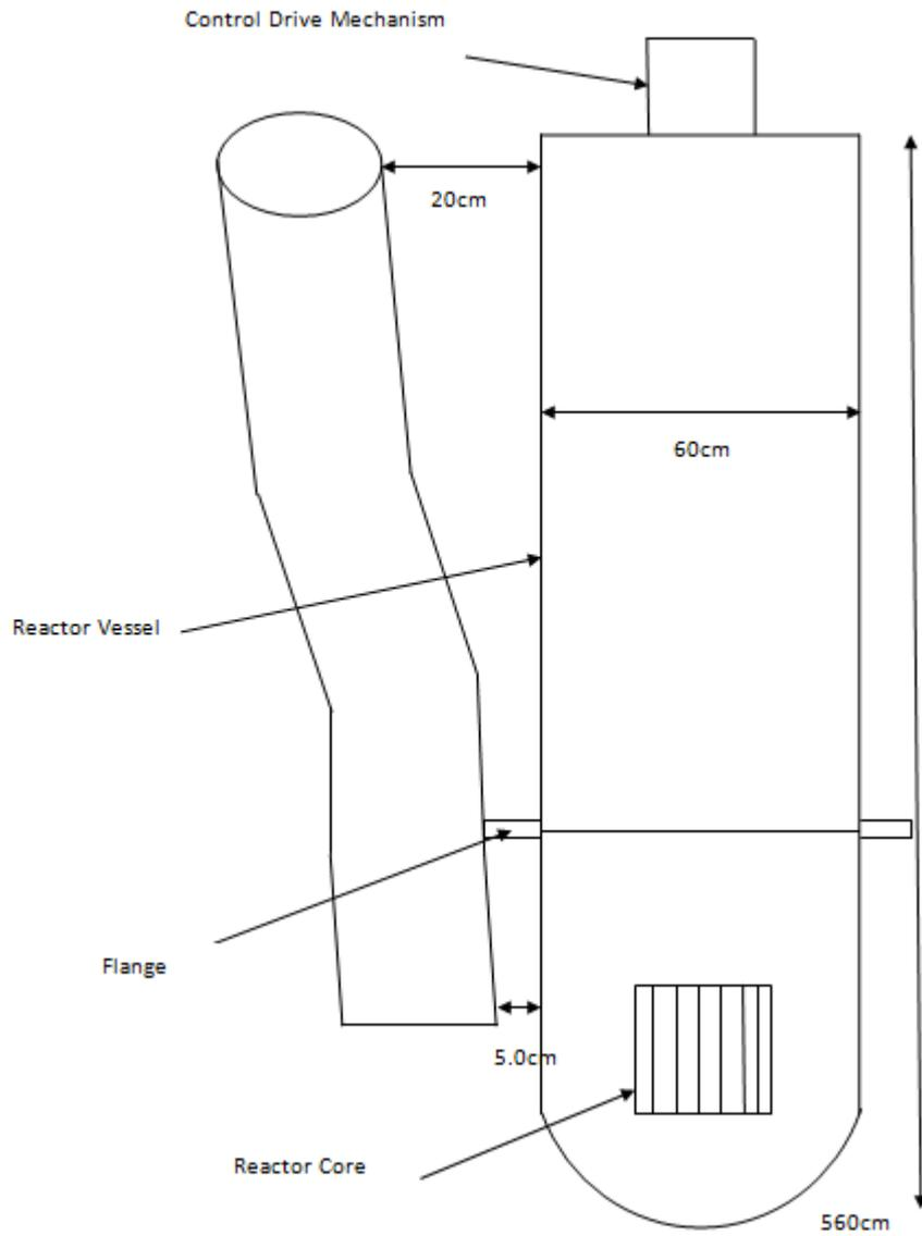
Figure 4.7. Vertical cross section of the reactor showing the slant tube
