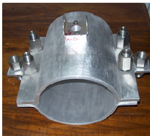
Fig. 12 Split type encirclement clamp
