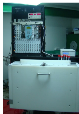
Fig. 9b System Control Electronics and Detector
