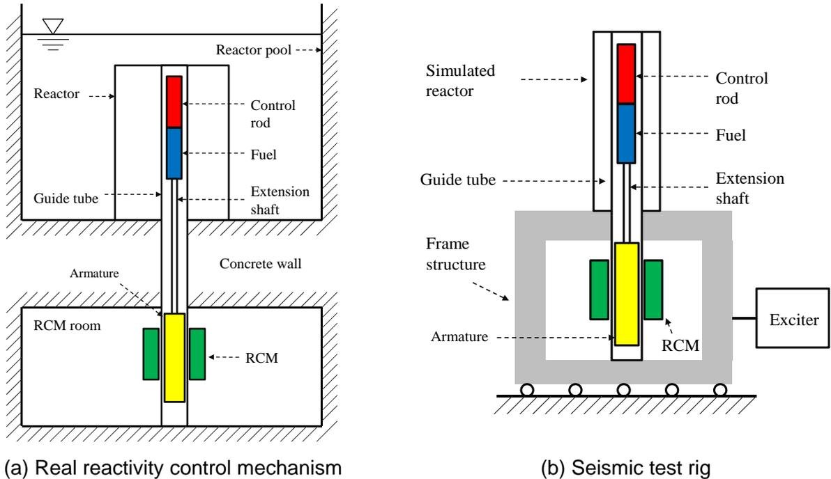
Fig 1. Schematic diagram of the reactivity control mechanism and its seismic test rig
