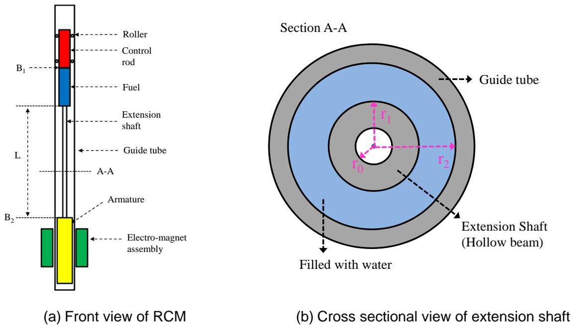
Fig 2. Schematic diagram of RCM
