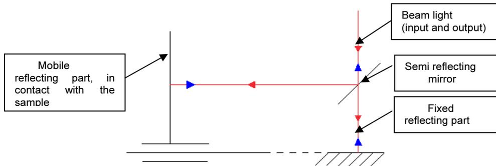
Fig 5. Principle of swelling measurement
