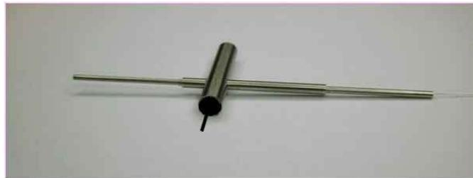
Fig 6. Optical module of the sensor inserted in device with a piston simulating the feeler piece
