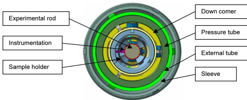
Fig 2. view of a sample holder and the test section (preliminary design)
